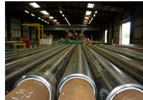
Dry insulation (PiP)
