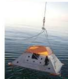
ADCP (Acoustic Doppler Current Profiler)
